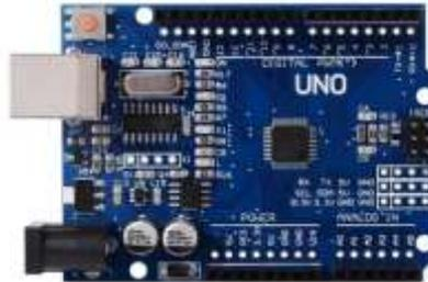
Gambar 1. Board Arduino Uno
