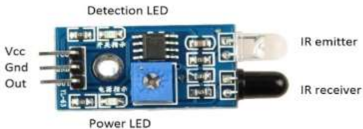
Figure 3. Sensor Proximity fc-51
