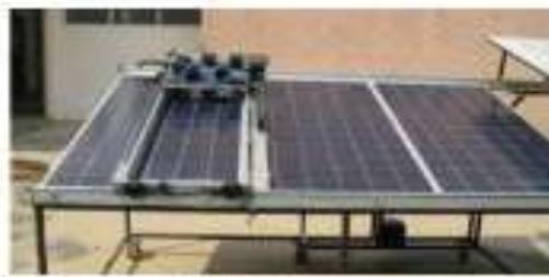
Figure 2. Solar Panel Cleaning Robot [3]
