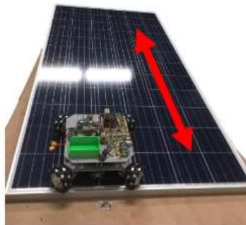
Figure 4. Roof Solar Panel Cleaning Robot
