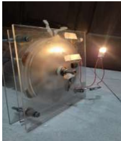
Figure 7 Testing a 1-Phase Axial Flux Generator with a Star-Shaped Stator and a Load
