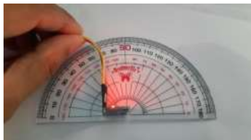
Figure 10. Gyroscope Sample Roll Angle Calibration Utilizing a Protractor
