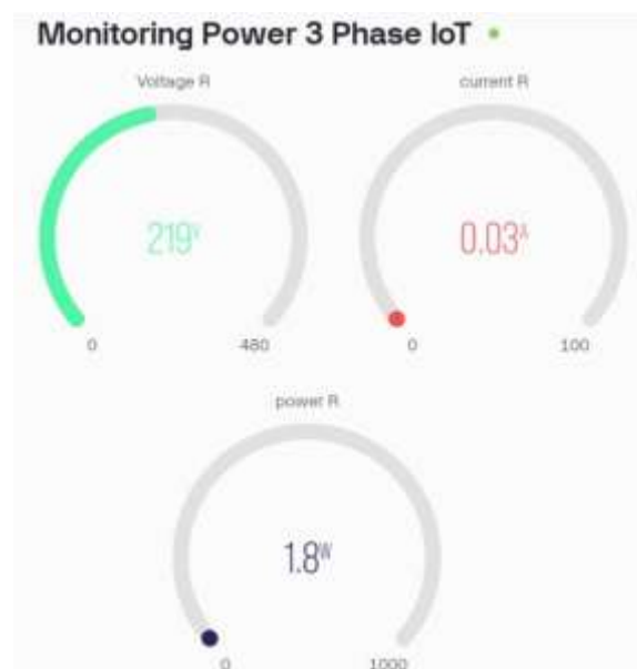
Figure 5. Measurement Results Displayed on the Blynk Application
