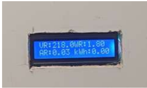
Figure 6. Measurement Results Displayed on a 16x2 LCD
