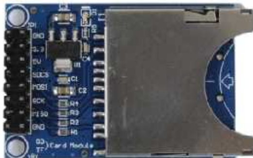
Gambar 4. Modul SD Card
