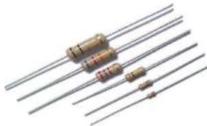
Gambar 3. Resistor Karbon
