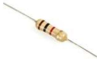
Gambar 4. Resistor Film Karbon
