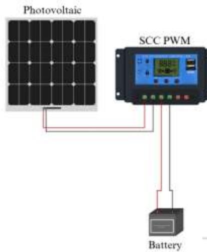
Figure 10. Hardware Circuit Wiring Without Peltier
