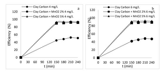
Figure 4. Adsorption efficiencies based on various types of adsorbents to contact time at the concentration of  $Pb^{2+}$  ion (a) 4 mg/L and (b) 6 mg/L
