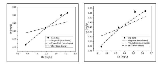
Figure 5. Model of Pb<sup>2+</sup> (non-linear) metal adsorption isotherms on (a) clay-carbon monolith adsorbents and (b) modified clay-carbon-manganese 5%.
