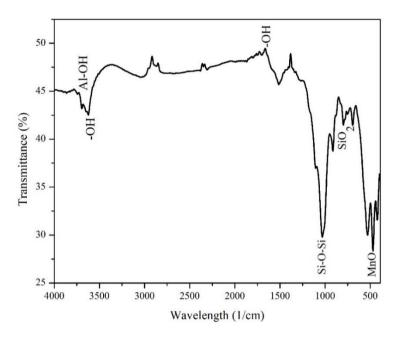
Figure 1. IR spectra of clay-carbon-manganese monolith before adsorption
