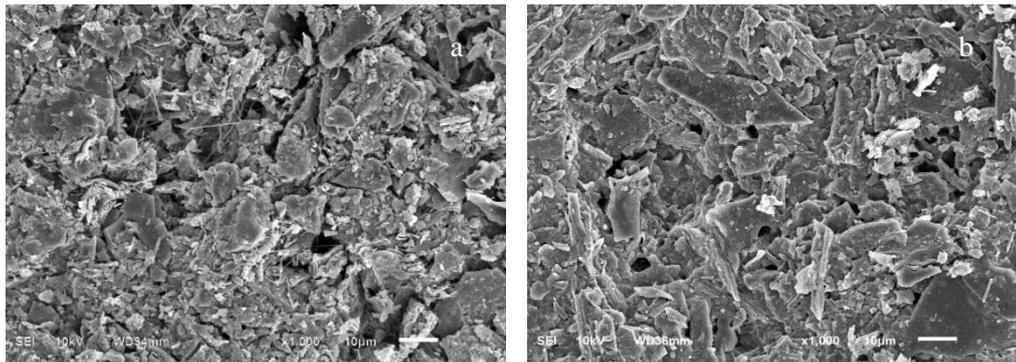
**Figure 3.** SEM results with 1.000x magnification of clay-carbon-manganese monolith adsorbent (a) before adsorption and (b) after adsorption
