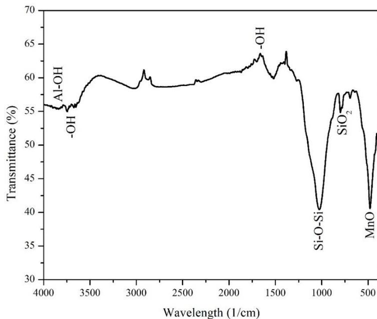
**Figure 2.** IR spectra of clay-carbon-manganese monolith after adsorption
