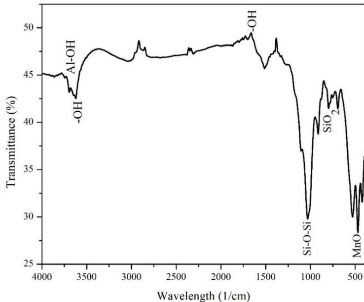
**Figure 1.** IR spectra of clay-carbon-manganese monolith before adsorption
