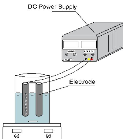
**Figure 1.** Batch system electrocoagulation
