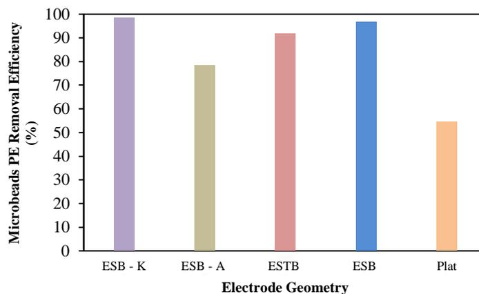
**Figure 4.** Effect of Electrode Geometry on the Removal of Microbeads Polyethylene
