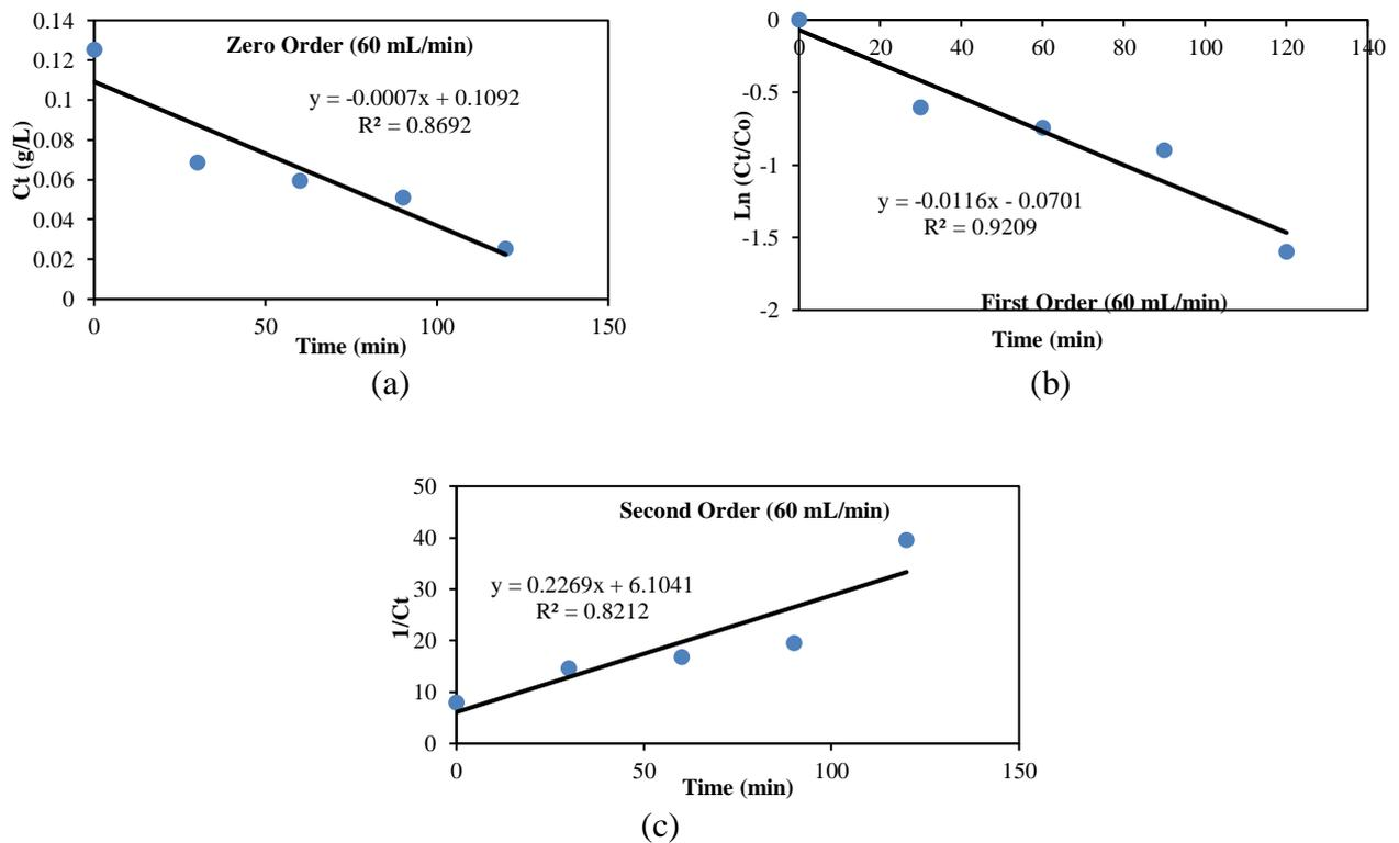
**Figure 10.** Kinetics reactions of microbeads polyethylene removal (a) zero order (b) first order (c) second order
