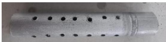
**Figure 9.** Effect of cathode after 120 minutes (flow rate: 90 ml/minute)
