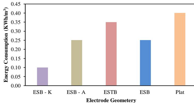
**Figure 6.** Energy Consumption Based on Electrode Geometry
