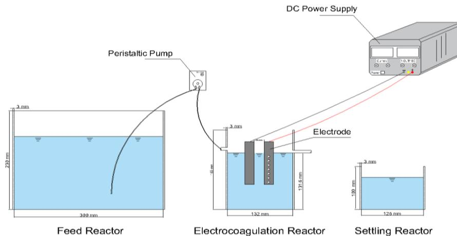
Figure 2. Continuous system electrocoagulation
