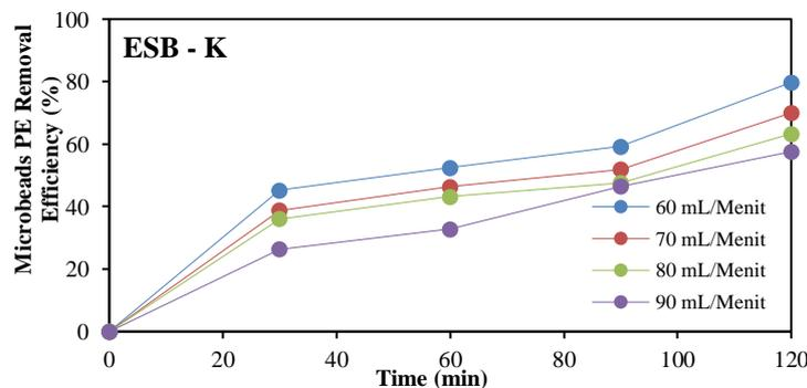
**Figure 8.** Effect of sample flow rate using ESB-K electrode geometry on the removal of polyethylene microbeads
