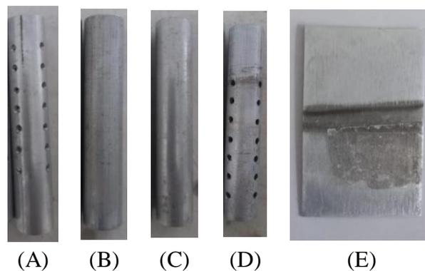
**Figure 7.** Passive Layer Formation on Aluminum Electrode Geometry (A) ESB-K (B) ESB-A (C) ESTB (D) ESB (E) Plate
