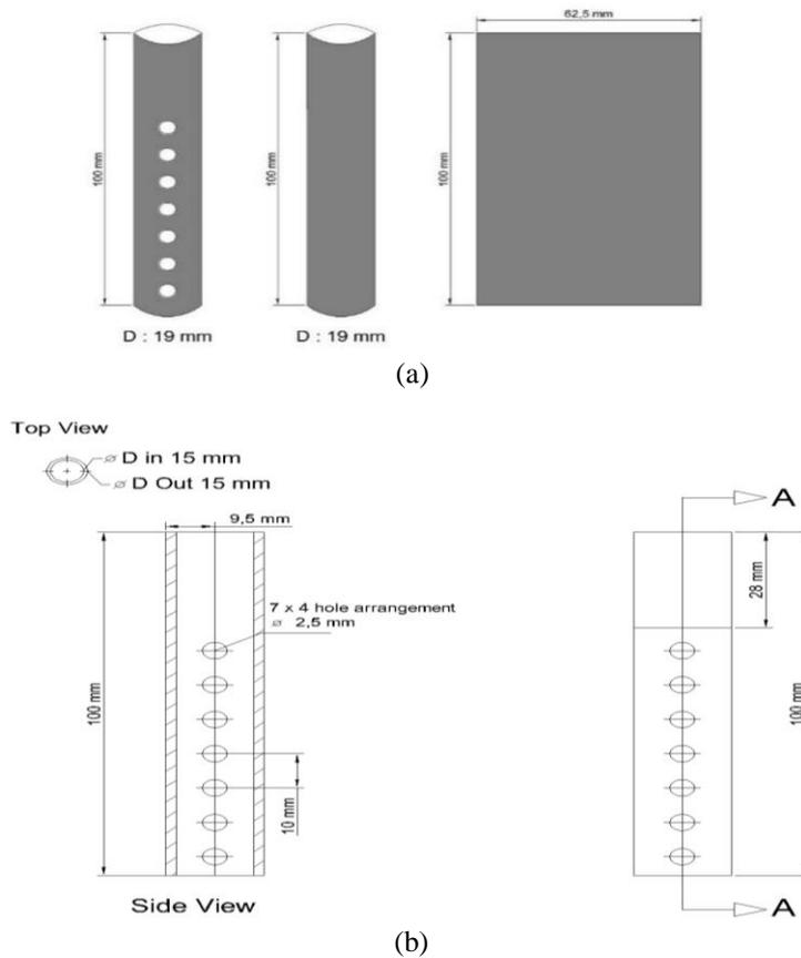
**Figure 3.** Schematic diagram of (a) the electrode geometry used and (b) details of the perforated electrode geometry
