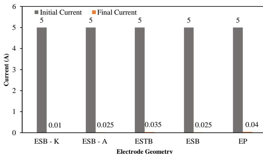
**Figure 5.** Initial and Final Current Strength of Different Aluminum Electrode Geometries
