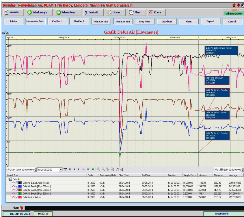
Figure 1: SCADA Distributed Water Graphs during April 2014
