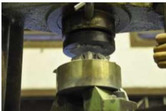
**Figure 6.** Compressive strength test for the mortar samples
