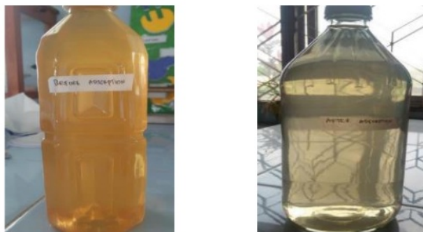
Figure 3. The colour of well water before (left) and after (right) adsorption using a biosorbent derived from areca fiber waste
