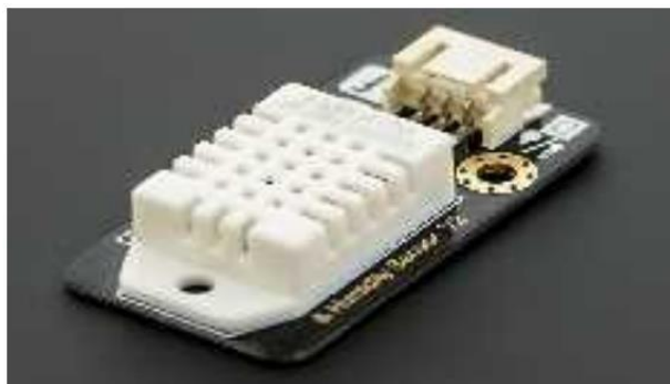
Gambar 4. DHT22 Sensor Suhu dan Kelembaban (Wijaya, 2016)
